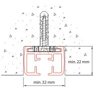
recessed mounting to or in ceiling with bracket
