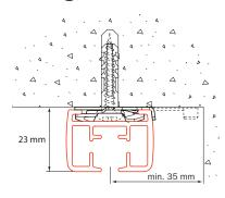
ceiling mounting with ceiling mounting clamp 6050: leave space to accommodate rotation of ceiling mounting clamp
