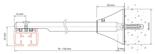
wall mounting with extension bracket 6017, can be cut from 15 to 7 cm
